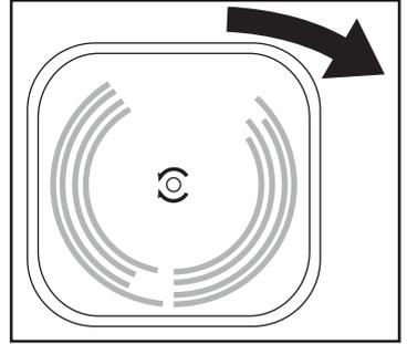
3. Replace the battery cover by fitting the center plastic column within the base and then twisting the cover clockwise until it clicks firmly into place.
