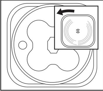
1. Turn the lantern over and remove the battery cover by twisting the cap counterclockwise.
