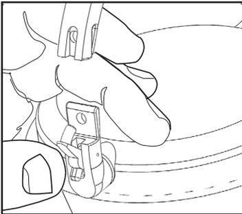
1. To open the handle, depress the raised button near the bottom of the handle.
